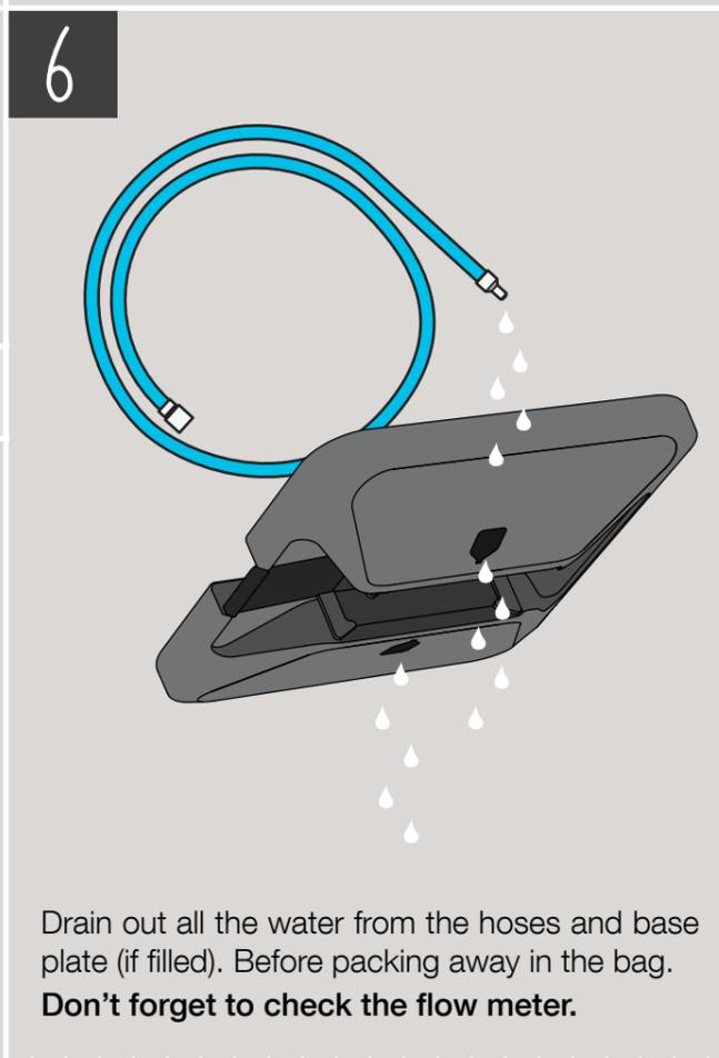
Drain out all the water from the hoses and base plate (if filled). Before packing away in the bag.
