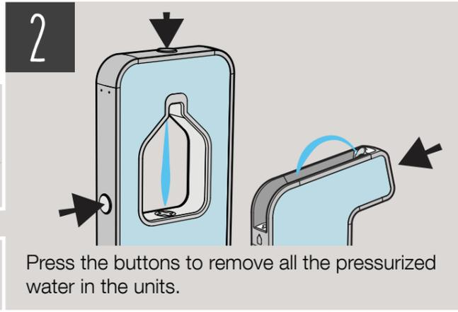
Press the buttons to remove all the pressurized water in the units.
