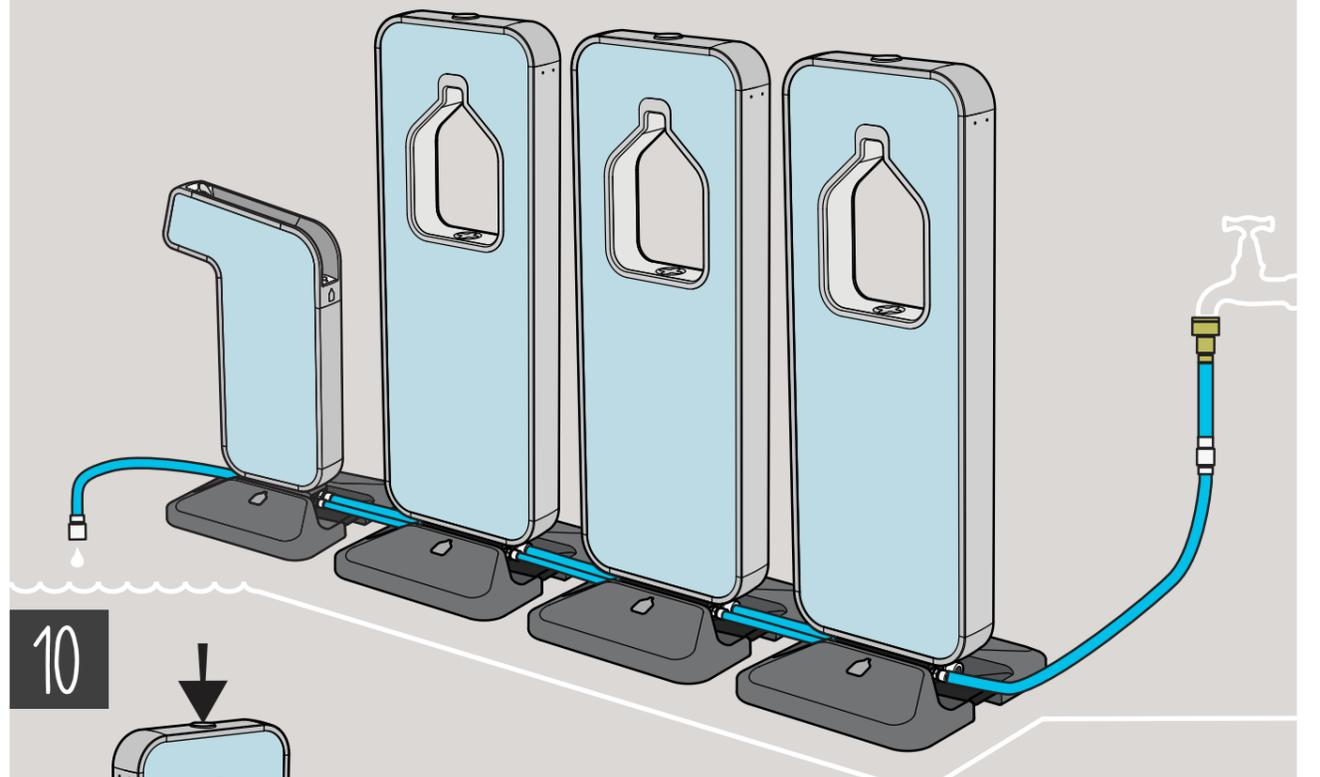
**10** Press all the buttons to flush out any air bubbles and old water in the lines. Run all the taps for 10 seconds. Check for leaks. If a leak is found turn off the water and check connections.
