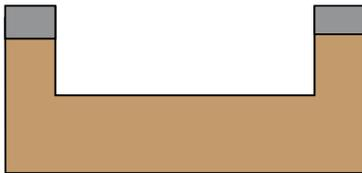
Excavate a hole in the ground. Recommend minimum footing size of 600W x 1100L x 550mm. This may need to be increased or reinforced depending on sub surface conditions. Plumbers to advise.
