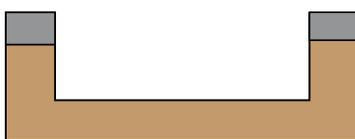
Excavate a hole in the ground. Recommend minimum footing size of 550W x 550L x 200mm. This may need to be increased or reinforced depending on sub surface conditions. Plumbers to advise.
